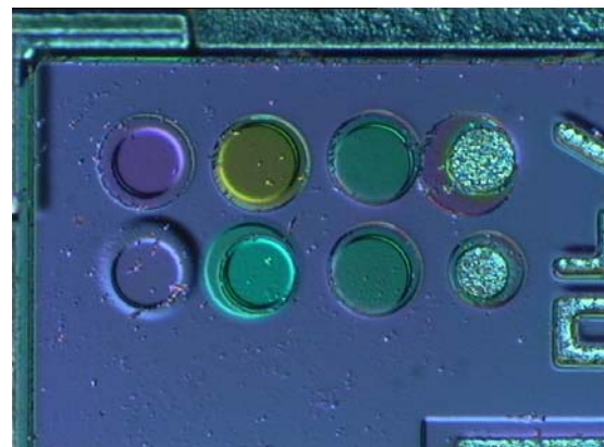
• Halbleiter, bright-field with differential interference contrast DIC, 50x Plan-Fluor.
